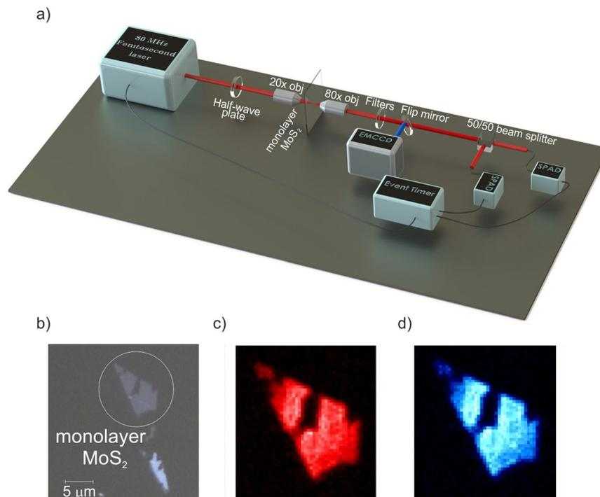
**Figure 1.** (a) Schematic experimental setup, (b) optical microscope image of mechanically exfoliated crystals (c) photoluminescence signal from monolayer MoS<sub>2</sub> measured with bandpass filter centred around 700 nm and (d) second Harmonic Generation (SHG) from the same monolayer crystal measured with a band-pass filter centred around 393 nm.
