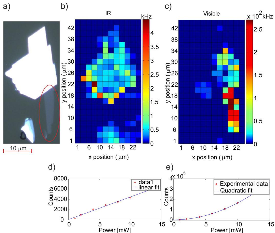
**Figure 3.** (a) Microscope image of the crystal. The monolayer region is indicated by the red oval, (b) IR signal intensity (counts) from the monolayer and bulk crystal, (c) SHG signal intensity (counts) from a monolayer and a bulk crystal of MoS<sub>2</sub> with 2 μm resolution. The pump wavelength for both SHG measurement in the visible and measurement of IR signal is 780 nm, (d) Pump-power dependence of the IR signal, (e) Pump-power dependence of the SHG signal.
